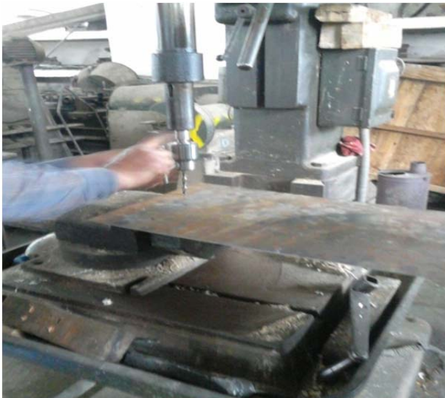
Fig. 2.2.3: Drilling of bolt holes
