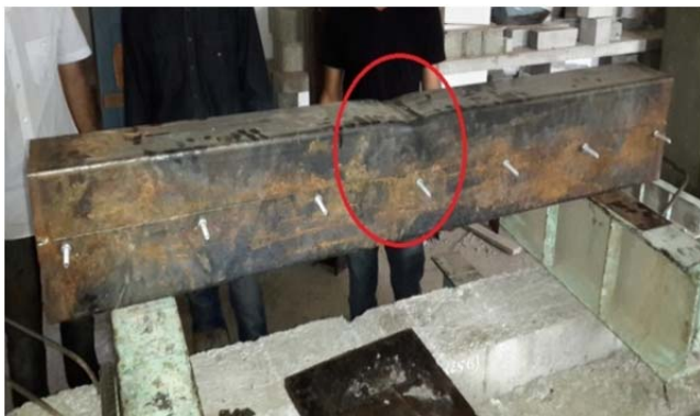
Fig. 3.2.1: Failure of Box Section
