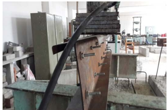
Fig. 3.1.1: Failure of I beam made of two channels
