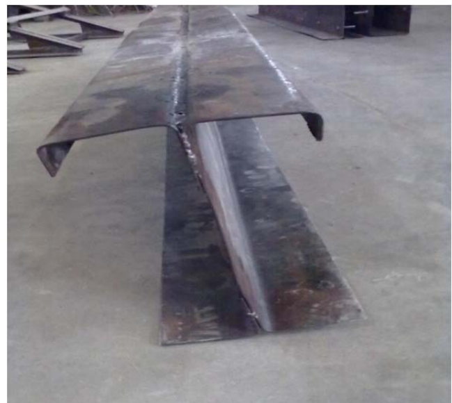
Fig. 3.3.1: Failure of I beam made of a channel and two angles connected to channel
